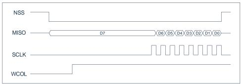
In addition, in slave mode, after writing the SPDR, the host-controlled NSS does not immediately become low. When the NSS is low, you need to wait for the second edge of the SCLK to start before entering the real data transfer state.
